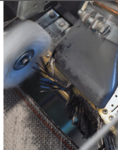
Fiber residues are extracted during the ongoing production process.
