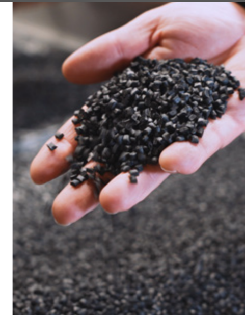
Example –WIPAG: thermoplastic compound (PP or PA) with 10 to 40 % carbon fiber content.
